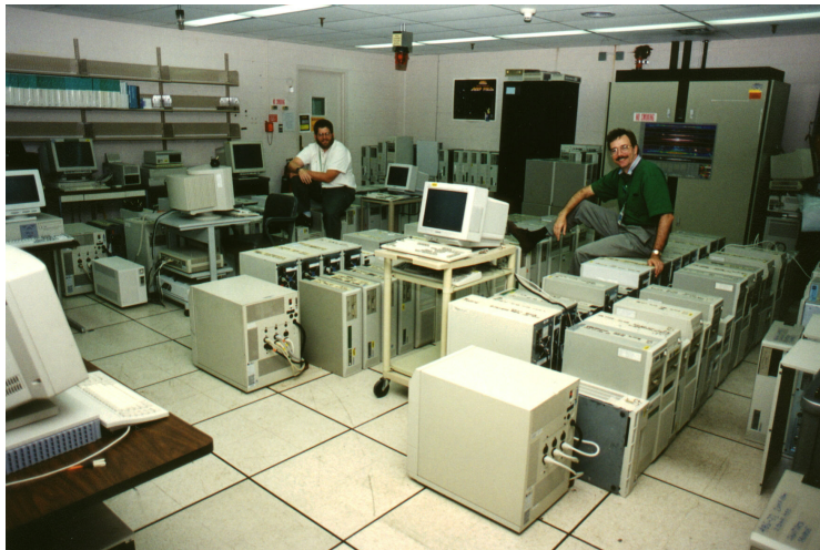
Figure: Originally developed in 1996–1997 for use on the Stone Soupercomputer, a very early Beowulf-style cluster constructed entirely out of surplus parts (see “The Do-It-Yourself Supercomputer”, Scientific American , 265 (2), pp. 72-79, 2001.)
