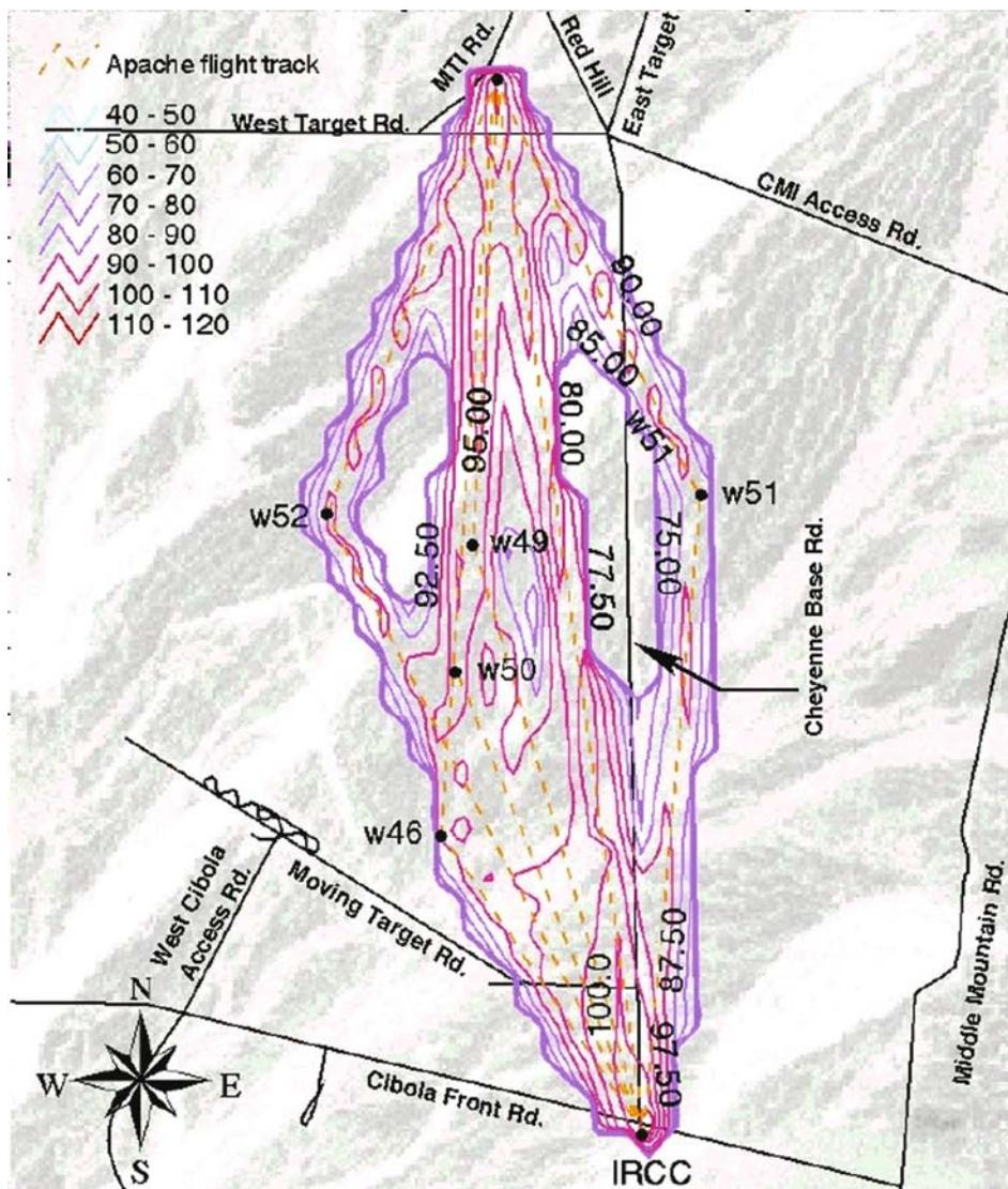
**Figure 3.** A-weighted decibel sound contours in Sound Exposure Level (SEL) metric, produced using NOISEMAP software, draped over Landsat 7 image of study site. Waypoint designations are marked with “w.” See Table 2. IRCC = Inverted Range Control Center.
