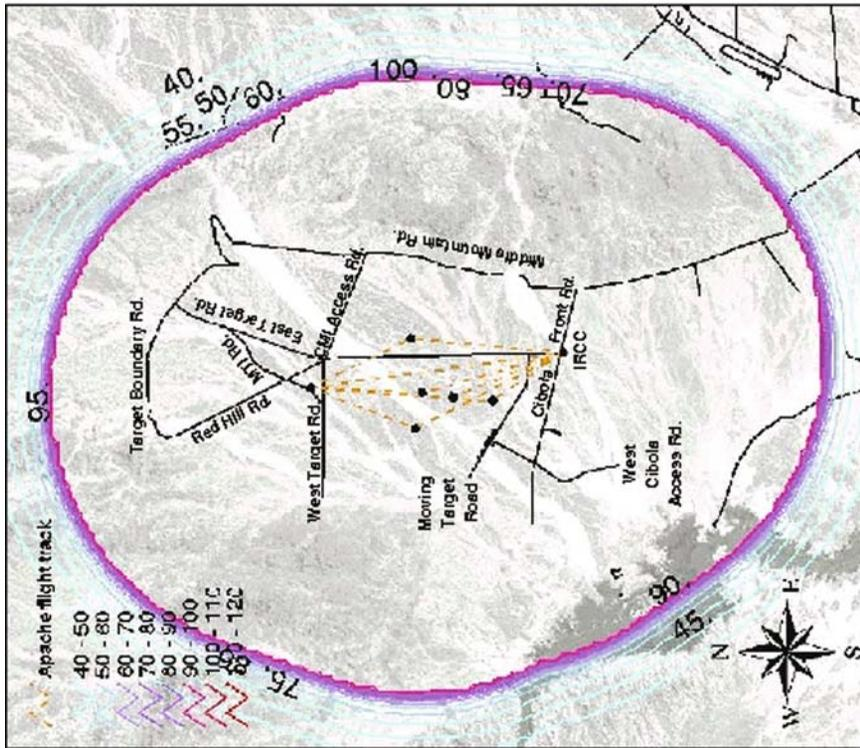
**Figure 2.** A-weighted decibel sound contours in Sound Exposure Level (SEL) metric (A) and  $L_{max}$  metric (B), produced using MR\_NMAP software, draped over Landsat 7 image of study site. Waypoints where the aircraft changed course are marked. IRCC = Inverted Range Control Center.
